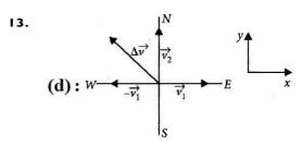
Velocity towards east direction,  $\vec{v}_1 = 30 \ \hat{i} \ \text{m/s}$ Velocity towards north direction,  $\vec{v}_2 = 40 \ \hat{j} \ \text{m/s}$ Change in velocity,  $\Delta \vec{v} = \vec{v}_2 - \vec{v}_1 = (40 \ \hat{j} - 30 \ \hat{i})$
